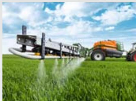
Due to the specific profile design, AMAZONE booms are at the same time superbly light and superbly strong. The working widths of the booms of 21 to 40 m allows the optimum matching to farm sizes and structure.
