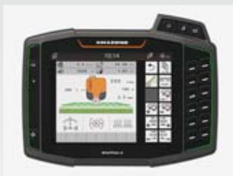
The AmaTron 4 operator terminal supports, for example, the precise switching in 50 part-width sections, automatic boom lowering at the start of application, automatic documentation and the part-area, site specific application rate control.
