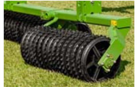
The AW rollers are available with either Cambridge or Crosskill rings in all working widths. The individual roller segments with their freely moving intermediate rings are mounted separately from each other in order to ensure outstanding self-cleaning and contour adaptation over the full working width.
