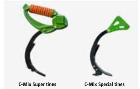
Together with the C-Mix Super pressure spring overload stone protection, the tine element in the centre of the machine provides a perfect working performance even when top soil deep loosening. In this way efficient and continuous operation is achieved even under the most arduous of conditions. The C-Mix Special tine with its shear bolt overload safety device is the alternative for light and medium-light soils without stones.
