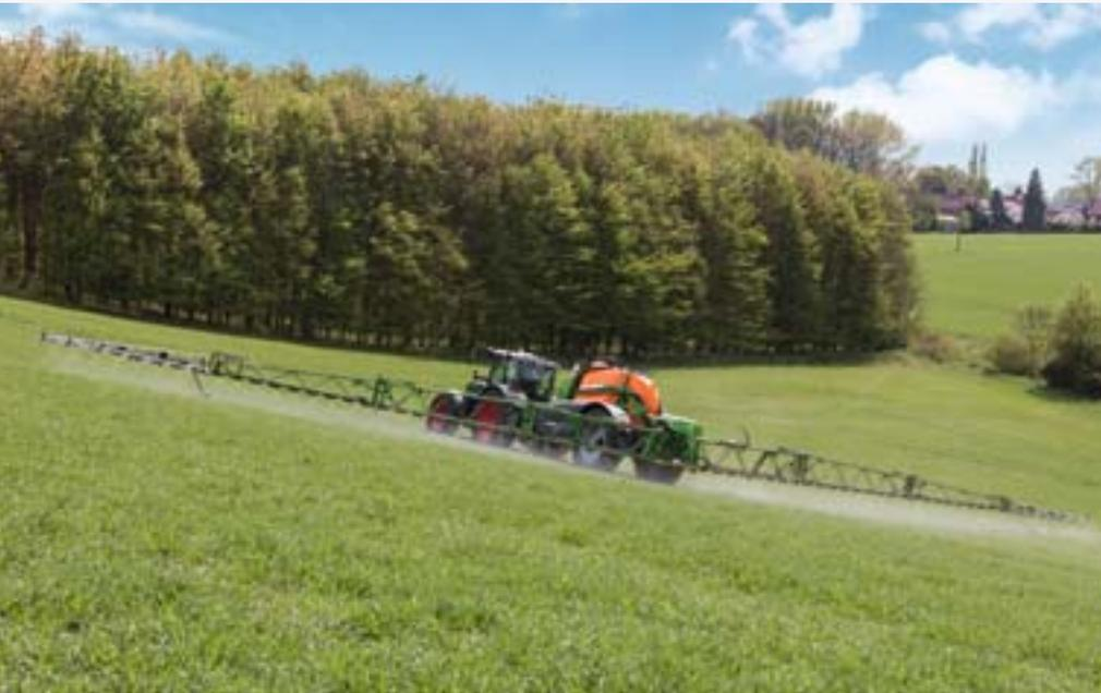
UX Super trailed sprayer with ContourControl and SwingStop
