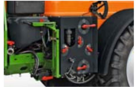
The clear control panel at the front left offers easy access for the fast, comfortable and error-free operation of all switches.
