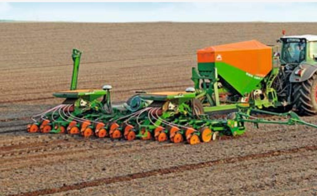
EDX 9000-TC trailed precision air seeder, 9 m working width
