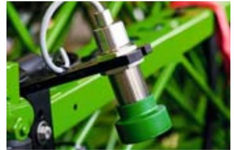
The DistanceControl plus boom guidance is equipped with four sensors. In addition to the increased number of sensors the regulating software now allows the optimum boom guidance even at higher forward speed and with reduced target area heights.
