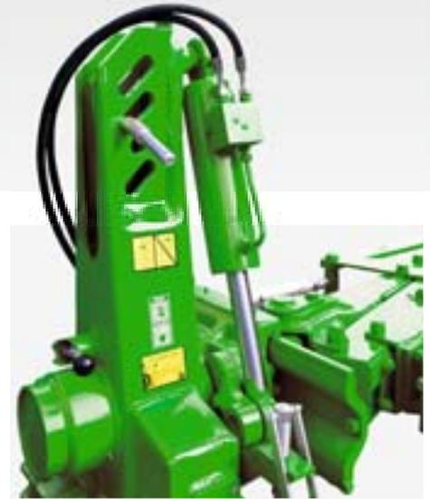
All headstocks on Cayros ploughs feature a turnover system that uses a double-acting cylinder with automatic changeover. This ensures that the turnover of the plough is smooth and jerk-free, plus it also means that the plough can be turned over using a single-acting spool valve with a pressure-free return as well. The hoses are optimally routed to prevent any potential damage.
