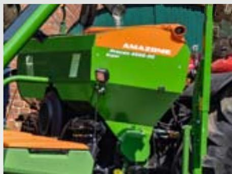
The fertiliser hopper can be installed with a capacity of 950 l or 1250 l depending on the model and level of equipment. The Precea-CC precision air seeder can be combined with Double-Shoot under-root fertilisation.
