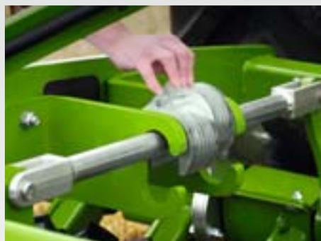
The working depth on the Catros Special can be comfortably adjusted by swivelling in and out spacer plates that are arranged centrally to the left hand side of the machine.
