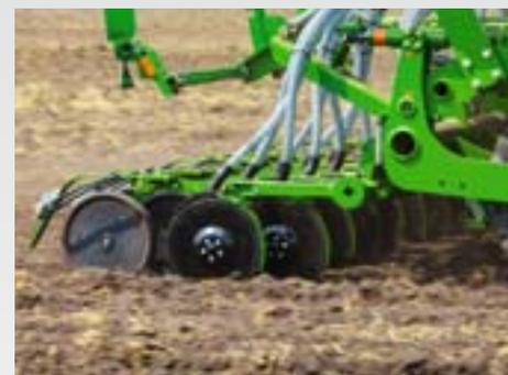
The TwinTeC+ double disc coulters system features an infinitely variable hydraulic adjustment of the coulters pressure providing a wide setting range from 15 to 100 kg. In this way, the pressure can be matched quickly and simply to the changing soil conditions.
