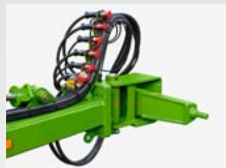
The Ceniux-2TX is coupled to the tractor via the lower links, a towing eye or a K80 ball coupling. This flexibility allows its use on tractors with caterpillar tracks or centre pivot steering as well its use on standard tractors.
