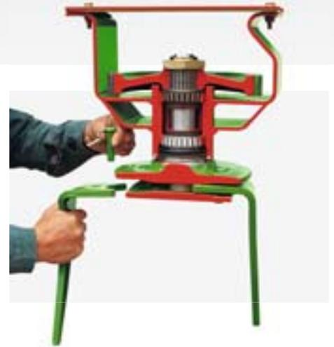
Quick change tine system for rotary harrows and rotary cultivators: The tines are simply pushed into the sockets of the tine carrier and secured with a lynchpin. There is no easier and faster way.
