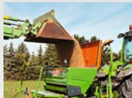
An especially-wide loading board, accessible via folding rear steps, simplifies the filling of the seed drill. The very spacious fill opening dimensions allow the quick and convenient filling process – not only from big bags and front end loader buckets but also from sacks.
