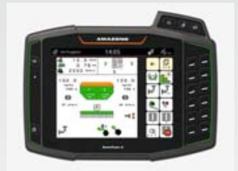
The AD-P can be operated via the AmaTron 4 and AmaPad 2 ISOBUS terminals or with any other ISOBUS compatible terminal, offering the possibility to equip the AD-P with GPS-Switch, the automated headland switch off system.
