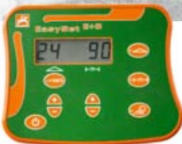
EasySet in cab operator terminal: for the electric operation of the shutter slide and spread width reduction
