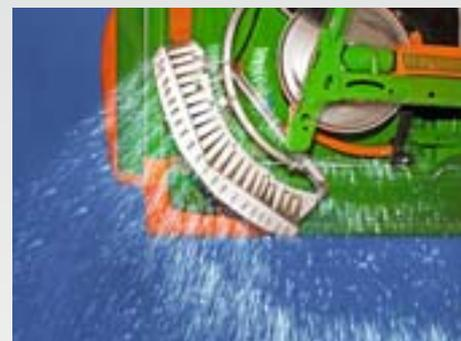
When side, boundary or water-course spreading using the hydraulically-actuated Limiter border spreading device, it is not necessary to either stop the spreading operation or to leave the tractor.
