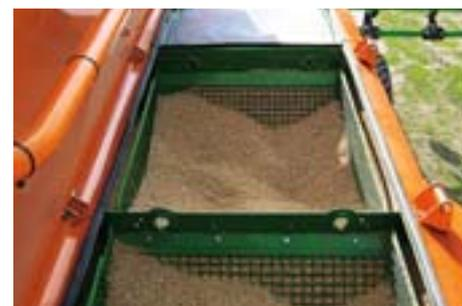
The pressurised tank, with a capacity of 8000 l, is divided into 2 sections (2/3 seed + 1/3 fertiliser). The fertiliser applied is transported with the seed into the seed furrow and in this way; for instance, when sowing winter corn, it is possible to apply an appropriate starter dose or when cultivating spring crops in drier conditions then the full optimum fertiliser quantity can be sown directly into the ground without losses.
