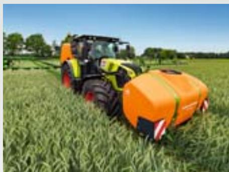
The tank shape was designed in such a way that both, on the road and also in row crops the view forward is not obstructed.
