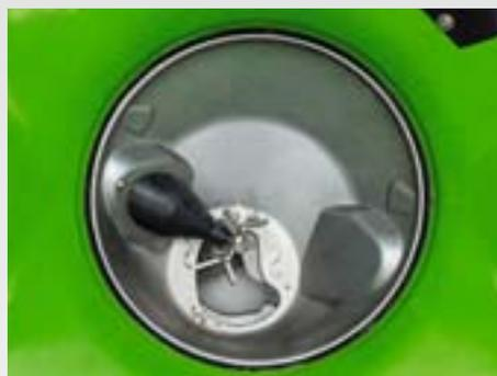
With the TS spreaders the electrically-driven star agitators in the hopper tips provide the even delivery of the fertiliser flow onto the spreading disc. They are automatically switched off, independently of each other, when either shutter is closed.
