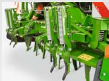
Optionally, for both rotary harrows and rotary cultivators the soil can be loosened in the tractor wheel marks with the height and side adjustable eradicator tines. The wheel mark eradicators are equipped with a sprung overload safety device to protect against damage.
