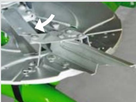
The TS spreading system with integrated, electro-mechanical operation of the AutoTS boundary spreading system – for normal and border spreading a different spreading vane is activated. This outstanding border spread pattern does not require a disc change – but is carried out remotely from the tractor seat during operation.
