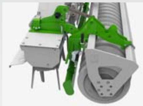
The levelling board levels the earth flow between the tines and the roller and presses the obstacles downwards. Where larger obstacles prevail, the integrated overload safety enables the levelling board to give way in an upward direction.
