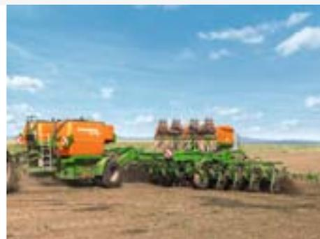
A FDC Fertiliser Delivery Cart can be used in combination with the Primera DMC seed drill, the Condor seed drill or the EDX precision air seeder, especially in dry farming locations. A pump transports the liquid fertiliser to the sowing coulters, which apply it to the soil. This combination is used to carry out sowing and starter fertilisation in a single pass.
