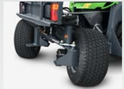
On the Profihopper SmartLine 4WDi, every wheel, due to accelerator pedal position and steering angle, is driven with the necessary speed for maximum traction. Especially in difficult operating conditions, the user benefits from the intelligent all-wheel drive.
