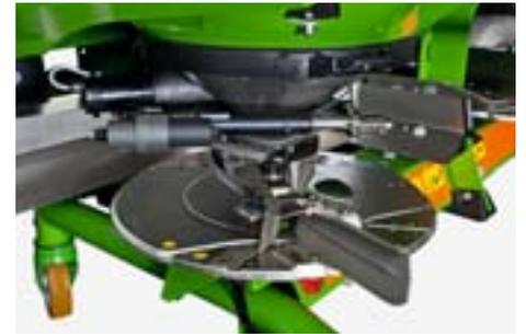
The delivery system, with the electrically driven agitator stars in the hopper bottoms, ensure an even fertiliser delivery onto the spreading disc. The slowly rotating, star shaped segments of the agitator evenly deliver the fertiliser to the relevant outlet opening.
