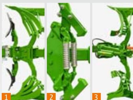
Three different stone safety systems are available from choice. A mechanical system via shear bolts (1), a half automatic release via coil springs (2) or a fully automatic hydraulic version (3).
