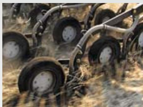
The ConTeC pro coulters excel themselves, because of the trailing guide wheel, with its precise contour following. The coulters spacing, the 3 stagger layout of the coulters and the high frame height guarantees a blockage-free operation.
