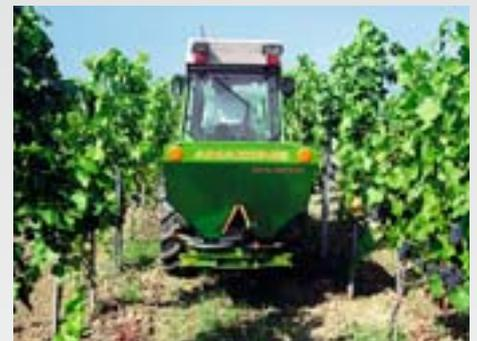
In the vineyard, the spreader's narrow overall width of just one metre prevents damage to the vines.
