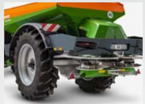
Over-sized tyres reduce the ground compaction and make operation possible even under the most difficult of conditions. Tyres with a cleated AS profile can be specified with a track width from 1.8 up to 2.25 m.
