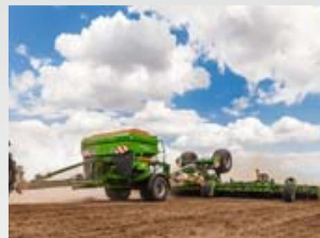
The trailed XTender-T is ideally suited to tractors without a three-point linkage or those with little lifting power. The running gear permits a support load from the attached implement of up to 4000 kg.
