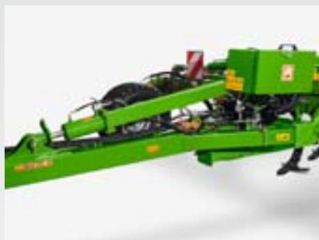
As an option, a selectable traction system is available. When activated, it additionally transfers part of the machine weight back on to the rear axle of the tractor with up to 1500 kg being available at a maximum working depth.
