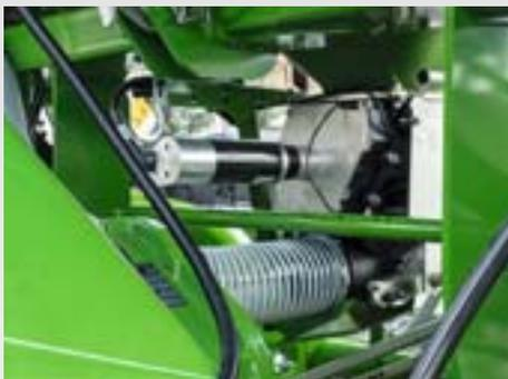
The seed metering is carried out via the electrically-driven metering unit underneath the seed hopper. When using different seeds, different metering cassettes are available which can then be quickly and easily exchanged.
