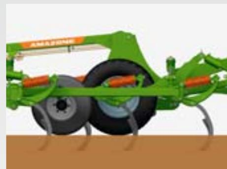
To ensure that the machine runs smoothly, also at the larger working widths, and operates at a constant depth, additional pressurised support wheels are integrated into the machine from a working width of 6 m. Again, to loosen the tracks of these wheels, a tine is also fitted behind each wheel.
