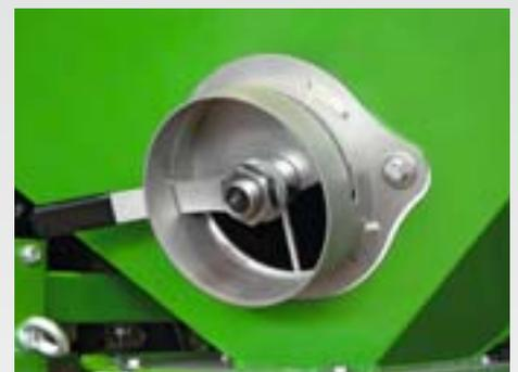
The emptying of the seed and fertiliser tanks is done quickly and easily via the optionally available quick emptying device which is attached to the tank and is easily accessible. By the use of some HT or drainage piping, the access can be extended to ease emptying.
