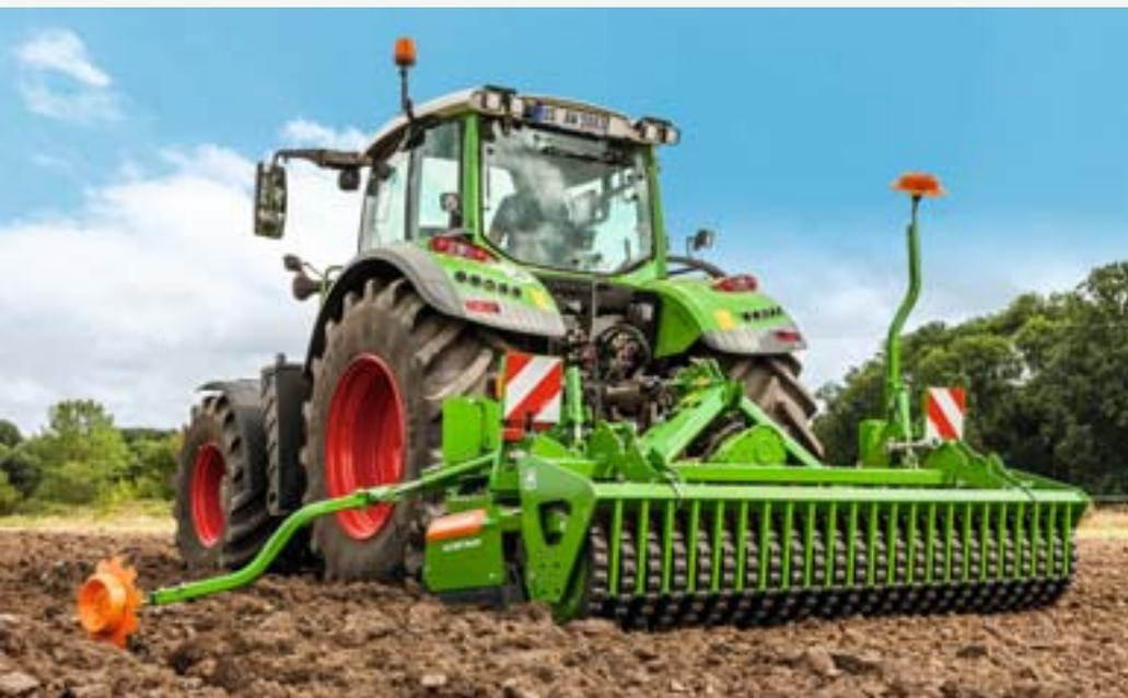
KG 3001 rotary cultivator with wedge ring roller with Matrix tyre profile
