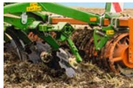
460 mm serrated levelling discs: ideal for working with large amounts of straw due to the increased mixing effect compared with smooth discs and so always a safe drive.
