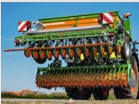
For transport or at the headlands the seed drill is pulled forward with the aid of the "Liftpack" system to reduce the lifting power requirement.
