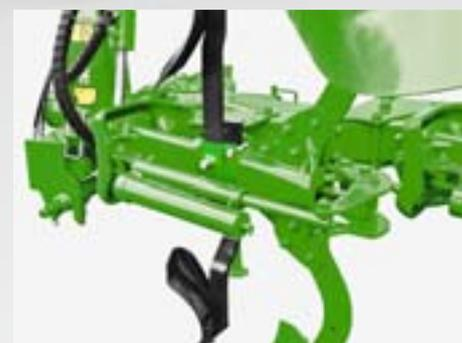
The hydraulic NonStop stone safety release features, in principle, one hydraulic cylinder per plough body with each one directly connected to a nitrogen-filled hydraulic accumulator. After having negotiated the obstacle, the plough body is automatically returned into position.
