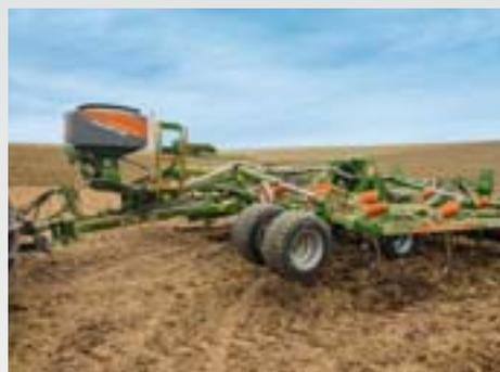
As special optional equipment for Ceniux-2TX, the GreenDrill seeder box is available. This allows the combined soil tillage and sowing of catch crops in just one operational pass.
