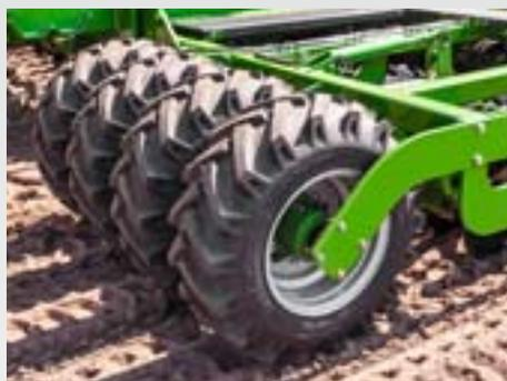
With the T-Pack S side packer, when using the Cirrus 4003-2/2C/2CC and 6003-2/2C/2CC under light to medium conditions or following the plough, the soil can be pre-rolled ahead of the disc segment, providing additional reconsolidation.
