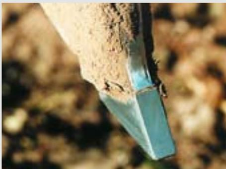
The hard-faced, “on-grip” chisel openers create a clean seed furrow into which the seed and fertiliser is placed – tried and tested 100,000 times over!
