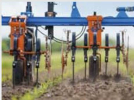
Hoe rollers protect sensitive crops from being buried by soil and guarantee optimum growth. Nevertheless, plants benefit from the additional nutrient mineralisation provided during hoeing.
