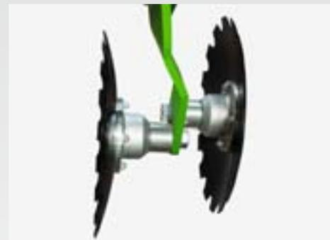
The 2-row disc harrow loosens, crumbles and levels the seedbed prior to the seed placement. The discs of the CombiDisc are aggressively angled, 14° at the front disc row and 12° at the rear disc row. This angle ensures the optimum levelling of the seedbed.
