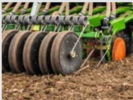
The Roller harrow additionally consolidates the soil above the seed furrow resulting in the optimum germination conditions. This is recommended especially for light, dry soils when sowing spring crops or rape.
