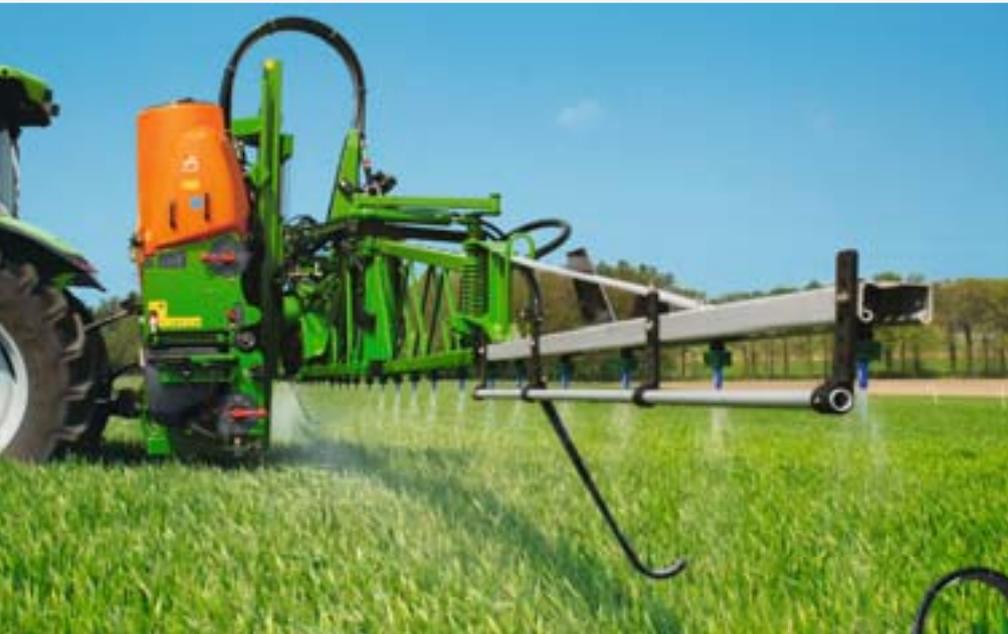
UF 1201 mounted sprayer with 18 m Super-S2 boom
