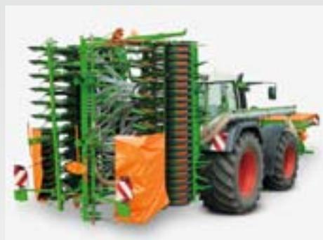
The Avant is available as rigid version in 4 m and in a foldable version up to 6 m which folds down to a transport width of 3 m for road transport.
