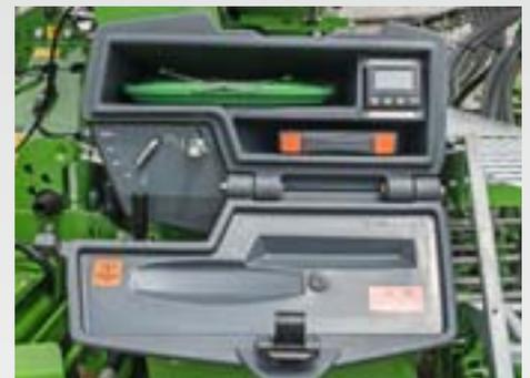
Via the SmartCenter, positioned to the left of the machine, the Centaya Super can be comfortably calibrated and adjusted from ground level. The digital weigh scales and a folding bucket are stored in the transport box to the side of the machine.
