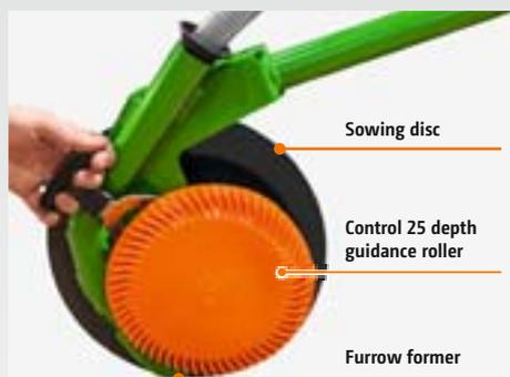
The RoTeC Control coulters, for sowing after the plough or mulch sowing, feature the Control 25 depth guidance roller enabling a tool-less and precise setting of the sowing depth.
