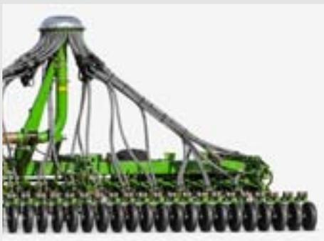
When the Citan is operated on dry soils, the HD roller harrow with hardened harrow tines is available. Independent from the sowing coulter, the following press rollers can be pressurised with 35 kg providing soil contact.
