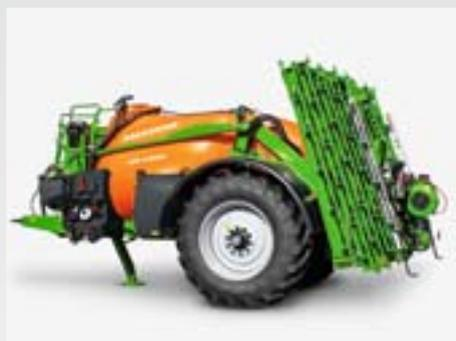
Alternatively, the Super-S2 boom, from 15 m to 28 m, can also be used on the UX. All booms can be automatically controlled with DistanceControl parallel to the target surface.
