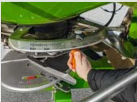
AMAZONE offers the ZA-V with both hydraulic and electrical shutter slide actuation. The hydraulic version allows the direct actuation of the shutter slides via two double-acting hydraulic spool valves on the tractor.
