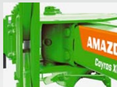
On the Cayros V, the setting of the furrow width is carried out steplessly and hydraulically from the tractor cab. Needless to say that the system is so sophisticated in design, that the traction point and the furrow width are also correctly adjusted at the same time.
