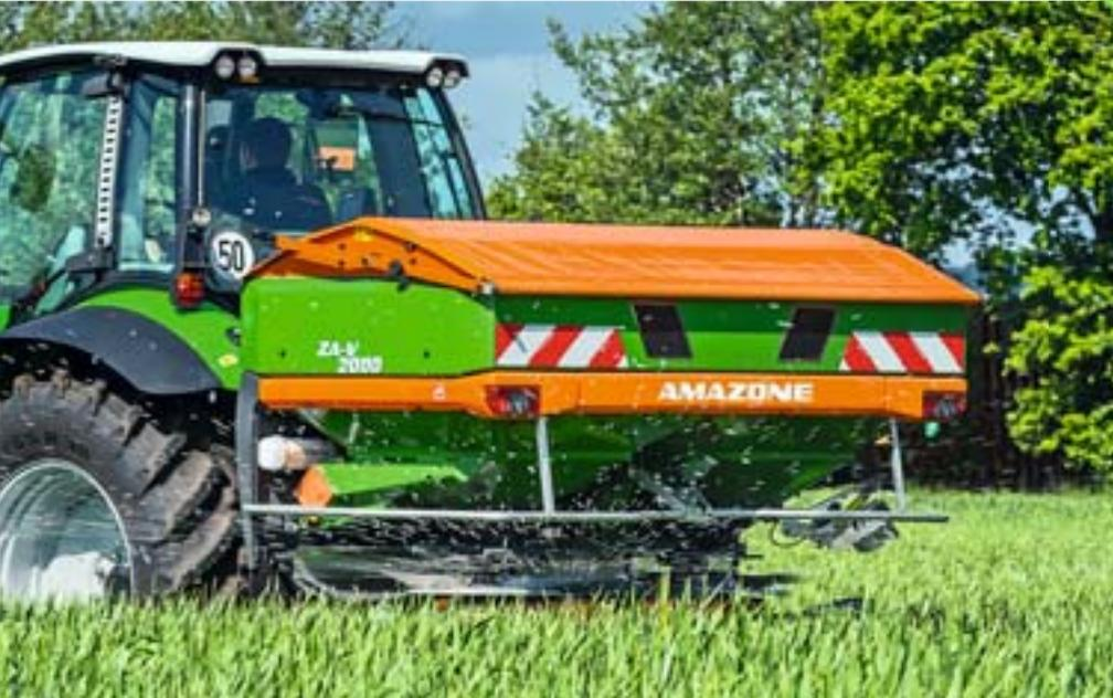
ZA-V 2000 twin disc fertiliser spreader
