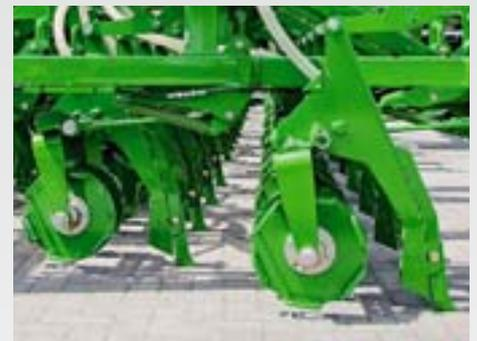
All the chisel openers are mounted on a parallelogram linkage. This prevents any reduction in the accuracy of the desired sowing depth even at different or changing forward speeds and in undulating ground conditions.
