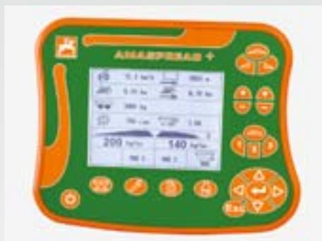
The AmaSpread+ in-cab terminal provides forward speed related spread rate regulation. The actuation of the Limiter V+ border spreading device, which can be fine-tuned between normal, side or border and water course spreading, is done via the push of a button directly from the tractor seat.
