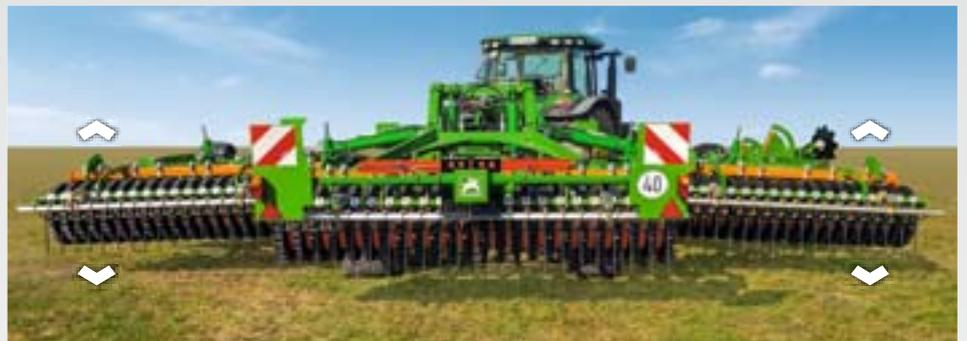
This perfect soil contour following ability is yet further enhanced by the ContourFrame system. Here, the hydraulic rams of the outer sections are pre-pressurised via hydraulic accumulators and then, when moved into the float position, it means that each of the three sections can adapt upwards and downwards to follow the soil contours – even in hilly terrain.
