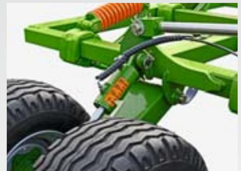
The optionally available step-less hydraulic depth control enables the adjustment of the working depth whilst on-the-move to react to varying soil conditions and operational conditions.
