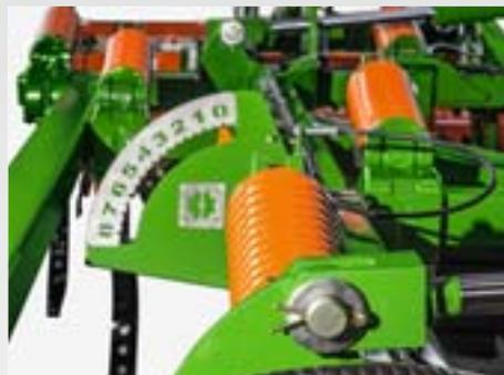
The optional hydraulic adjustment of the levelling unit means that the complete set-up of the machine is possible from the tractor cab. Using the clear scale, which is easily visible from the tractor cab, the current working position of the levelling discs is readable.
