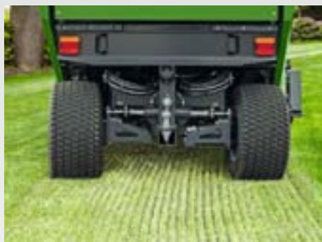
The Profihopper is also a superb scarifier. The scarifying knives, which are quickly attached without tools, slit the turf and thin out the lawn's surface. Thatch is removed, collected and at the same time the soil is rolled.
