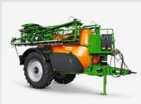
With a transport width of just 2.6 m, the Super-L2 boom, from 21 m to 36 m, folds down very narrow next to the tank. With a maximum transport height of just 3.8 m, the UX is very compact, even with high tyre sizes (18.4R46).
