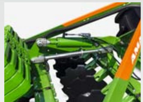
The hydraulic depth adjustment, which can be chosen as an option, offers huge comfort for the Catros and Catros Special. Changeable on the move, it allows the adjustment of the working depth from the tractor cab.
