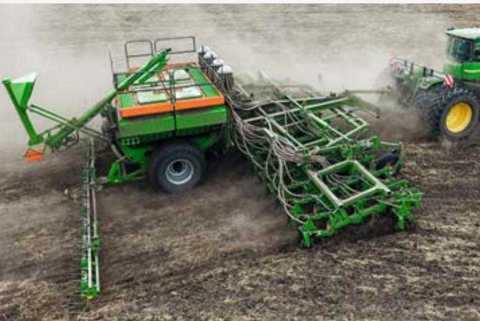
Primera DMC 12001-2C, 12 m working width with external distributor heads
