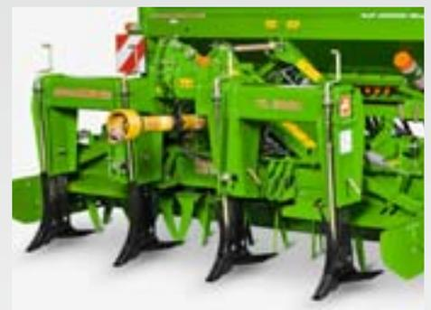
The compact TL deep loosener loosens and inverts the soil. This enables AMAZONE to offer one-pass cultivation without ploughing, even where high levels of straw prevail.
