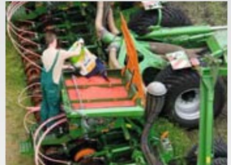
With a working width of 9 m yet only 2 seed hoppers have to be filled. This centralisation means shorter filling and set-up times and thus results in an additional increase in efficiency.
