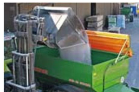
The large-volume tyres reduce pressure on the soil. The hopper can simply be filled from the silo or the loader.
