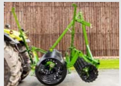
The optional NRP breaker ring roller is available as a following roller to give a more intensive levelling and crumbling effect.
