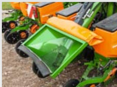
For filling the ED with fertiliser, AMAZONE offers a hydraulically-driven filling auger, integrated within the machine concept. In this way fill times can be reduced and the work rate of the machine further increased.
