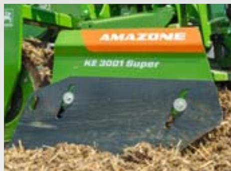
The side plates are mounted on a sprung suspension which allows them to yield upwards when stones are encountered. A long carrying arm and sturdy springs also make the KE Super reliable to use on stony, heavy soils. This applies also to all rotary cultivators.
