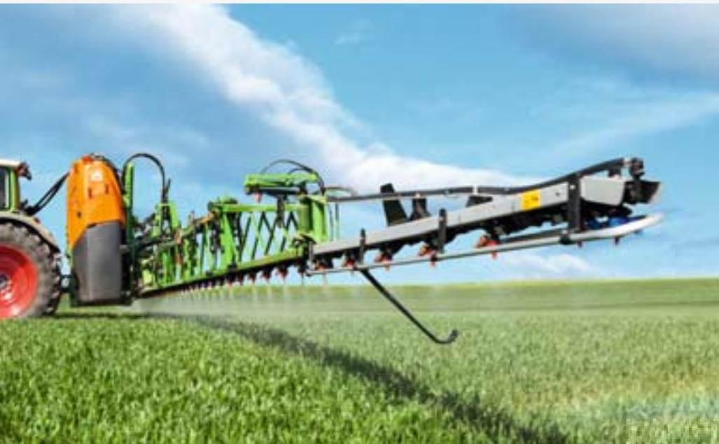
UF 2002 mounted sprayer with 30 m Super-S2 boom
