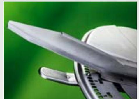
Only 3 pairs of spreading discs cover the entire operational range from 10 m to 36 m. The working width is simply, quickly and safely adjusted via the spreading vane position. Setting of the spreading vanes is carried out without any tools via the QuickSet adjustment system.
