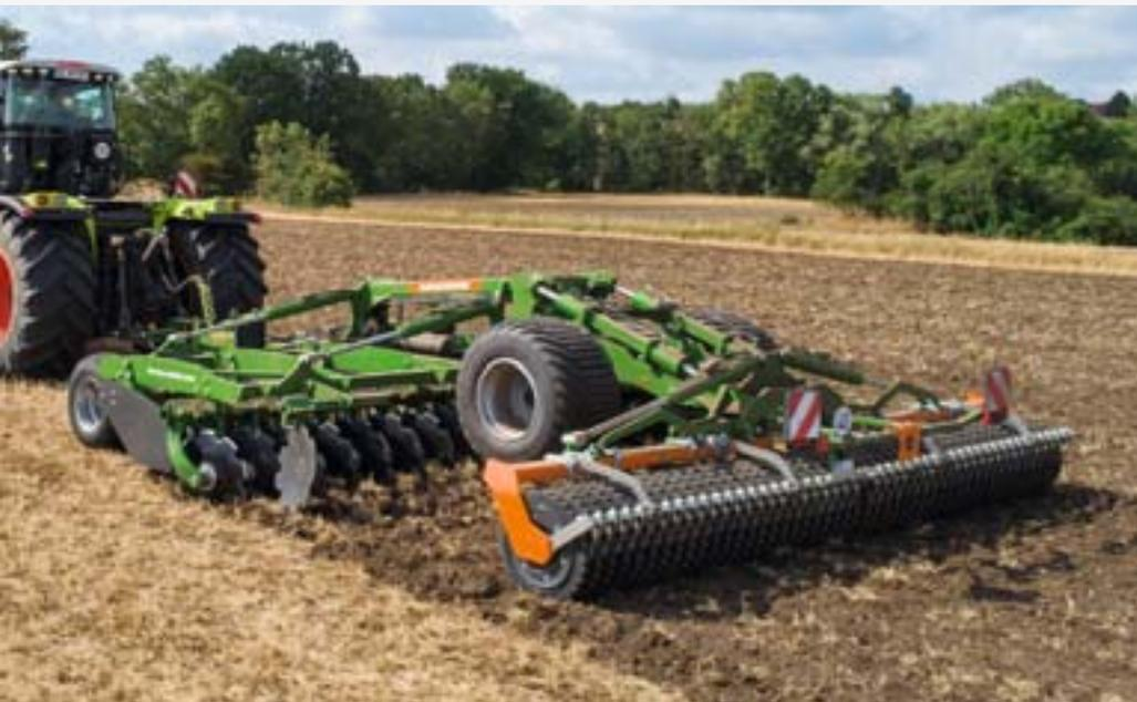
Certos 6002-2TX in 6 m working width with TX centre running gear in work
