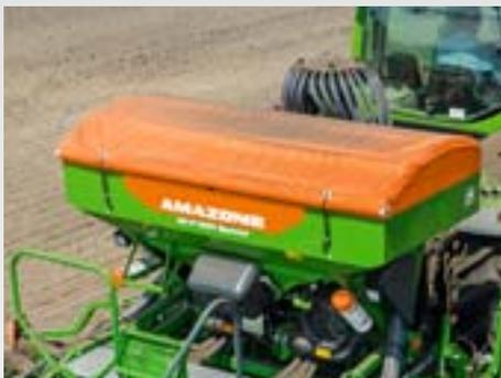
The roll-over hopper cover is easy to handle and protects the seed hopper from dust and rain.
