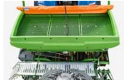
The hopper opening features a spacious 2.43 x 0.91 m so that the Centaya can be filled via big bags or via a front end loader without a problem. When filling via small sacks, the protective sieves in the seed hopper can be utilised as a loading aid.
