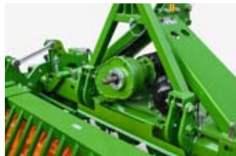
Via the PTO shaft through-drive, a mounted implement, for instance such as a pneumatic seed drill, can be driven.
