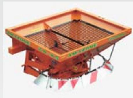
The ZA-XS H mounted spreader has been designed especially for road construction. Thanks to its hydraulic drive, this twin disc spreader is ideally suited for road rollers which simultaneously apply grit to the road.
