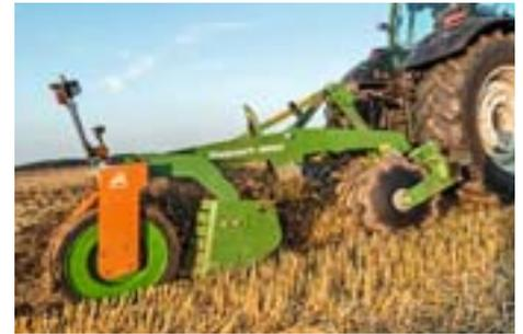
Due to the wide disc gang spacing, the Catros<sup>XL</sup> is characterised by its additional free passage of material. Thanks to the open frame construction with plenty of open space, the incorporation of catch crops, grain maize straw or potato haulm is possible without any problem in addition to stubble tillage.
