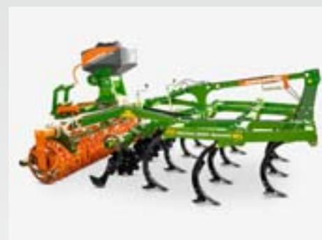
The mounted GreenDrill is available in working widths of 3 m, 3.5 m and 4 m. It is ideally suited for sowing fine seeds and catch crops.
