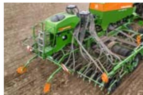
The pneumatic GreenDrill catch crop seeder box, when mounted on the trailed Cirrus sowing combination, allows the user to apply to the soil surface an additional medium during the sowing procedure. This could be in the form of either seed for under-sowing or for applying slug pellets.
