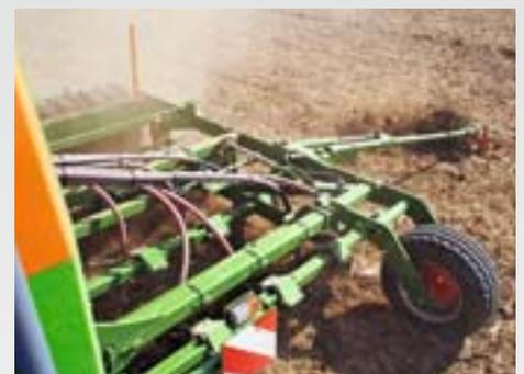
At 3600 l, the seed hopper on the Cayena is large, but still compact. This allows a clear view of the TineTeC coultters during use. The large hopper opening ensures the easy and rapid filling.
