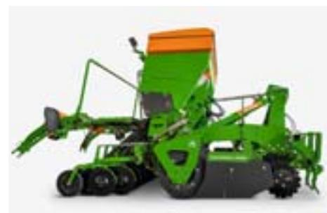
Thanks to the QuickLink quick coupling system, the CombiDisc can be removed with just a few hand clamps so that the mounted compact disc harrow can be readily used in solo operation for seedbed preparation.
