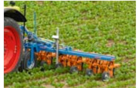
Precise camera and control technology leads to an enormous increase in output. Even row spacings as narrow as 12.5 cm can be detected by the camera. Thanks to the camera technology, driving speeds of up to 15 km/h are now possible without any problems.
