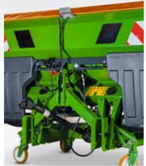
The weighing system offers controlled comfort as well as more peace of mind. With its 200 Hz weighing system, it works on-line to determine the different characteristics of the spreading material – and all this with the highest degree of measuring accuracy. It automatically compares the actual applied rate with the pre-determined rate.
