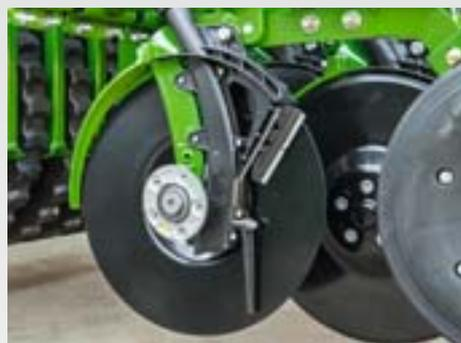
The Cataya Super catch crop seeder box is equipped with either RoTeC Control single disc coulters or TwinTeC double disc coulters.
