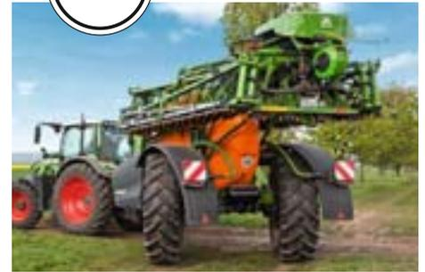
For the UX Super also a new steering axle with a maximum steering angle of 28° is available. Thanks to this big steering angle and the compact design of the UX Super, it can circumnavigate very tight curves. Depending on tyre size and track width, a minimum turning radius of 4.5 m is possible.
