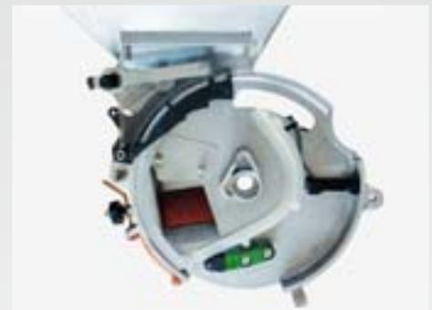
AMAZONE precision air seeders function according to the vacuum principle. The singling, on both the mechanically (ED Special) or hydraulically (ED Super) driven seeders, is carried out via a stripper finger.
