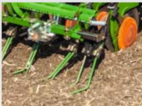
In order to cope with the ever-increasing sowing speeds, the RoTeC pro coulters feature an especially strong coulters bearing point. The Exact S following harrow provides good seed coverage, even under the most arduous of operating conditions and where copious amounts of straw prevail.
