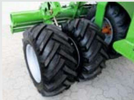
As an alternative for regions with are less sensitive to germination conditions, the Cirrus can also be equipped with a simple AS cross-ply tyre. The self-driving effect from its short cleats is very good and thus the machine is also easy to pull.
