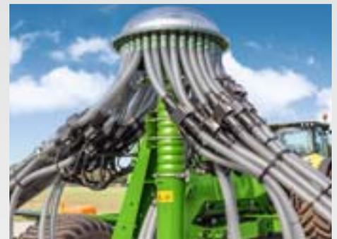
A useful system to assist the driver is the optionally available seed pipe monitoring which detects immediately any blockages down at the coulter and in the tube. Sitting directly behind the distributor head, sensors monitor the seed flow in the seed pipes.
