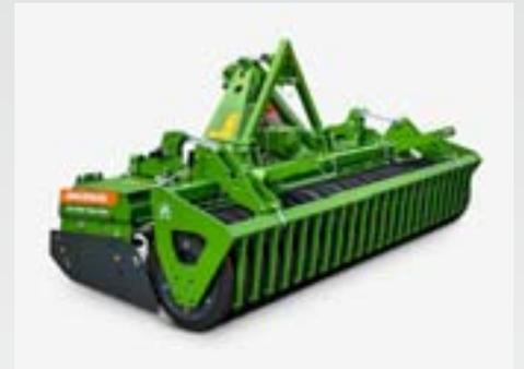
The unique wedge ring roller ensures reconsolidation in strips. The seed is placed in the strips. Suitable for all weather conditions and all soils.
