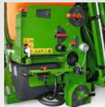
The operator station of the UF is located on the left hand side of the machine. Only three operating taps are sufficient for the actuation of all functions.
