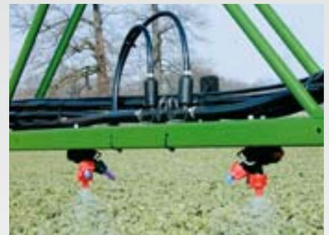
The pressure re-circulation system (DUS) for all AMAZONE sprayers ensures that the concentration of spray chemical at the nozzle is always constant. When cleaning, the system is flushed with clear fresh water right up to the nozzle.
