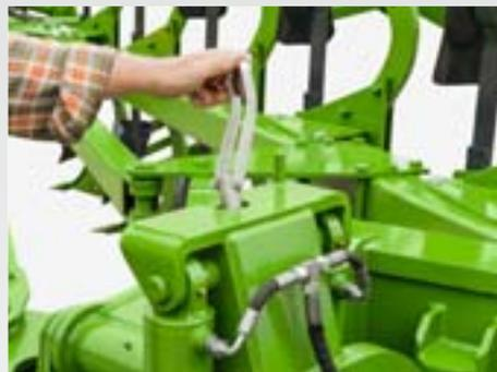
The working depth is set steplessly and without tools via the support wheel.
