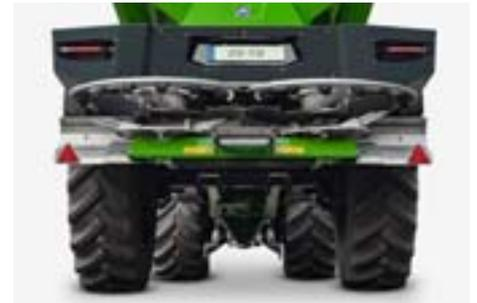
The sheet metal is manufactured from high-quality steel to withstand the abrasion caused by the fertiliser. The ZG-TS high-performance trailed spreader comes with a mechanical spreading disc drive, whereas the ZG-TS Hydro has hydraulically-driven discs.
