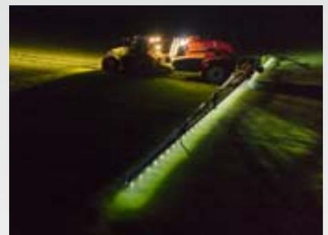
The optional LED individual nozzle lighting means that the illumination of the spray fan is targeted even more. Even the functionality of the last nozzle on the boom can be checked without a problem.
