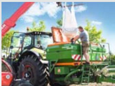
The XTender features a pressurised tank with a capacity of either 2200 l or 4200 l, which can be split in a ratio of 50/50. Application rates from 2 to 400 kg/ha can be achieved. Thanks to the large hopper opening, filling is quick and simple to accomplish.
