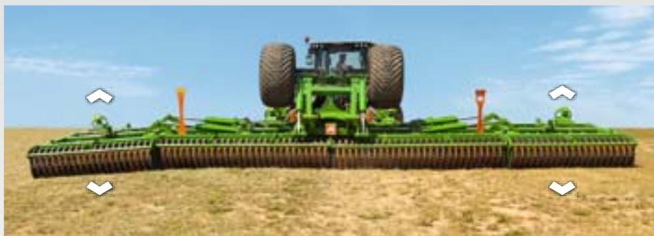
The Catros+ 12003-2TS comes equipped with 510 mm diameter serrated discs making possible working depths from 5 down to 14 cm possible. The ContourFrame on the Catros+ 12003-2TS is divided in four separate segments allowing each of them float. In this way the pressurised hydraulic system allows the individual soil contour following of each of the 4 segments.
