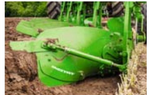
The X-blade widening share is a specific mouldboard extension mounted on the last plough body and creates, on average, a 30% wider furrow bottom.
