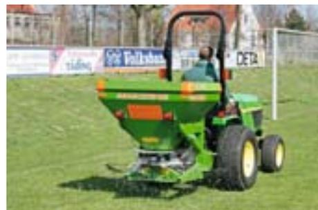
With minimal expense, the E+S winter application spreader can also be equipped for spreading granular fertiliser. It produces an excellent lateral and longitudinal spread pattern as well as achieving high work rates.
