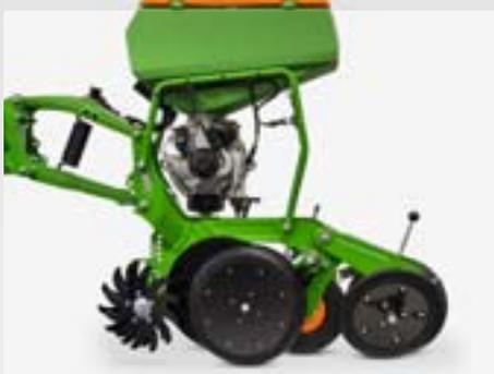
The PreTeC mulch seeding coulter has a maximum coulter pressure of 220 kg, using mechanical coulter pressure, and 400 kg using hydraulic coulter pressure. This ensures smooth running and even field emergence under the hardest of soil conditions.
