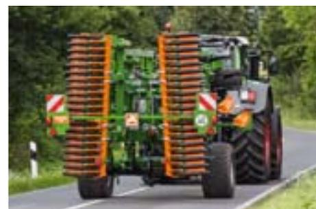
The integrated running gear provides the machine with a high manoeuvrability both, on the road and in the field. Depending on country-specific traffic regulations, an allowable 40 km/h fast road transport speed is possible.
