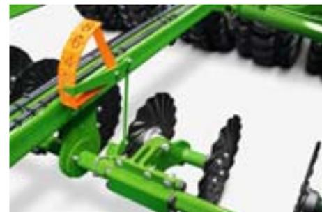
With the Minimum TillDisc corrugated disc segment, the Cirrus gets a new special option in place of the cultivation discs. On a row spacing of 16.6 cm, the ground, the harvest residues and also any green crop can be cut directly in front of the sowing coulters for a clean seed/soil contact.
