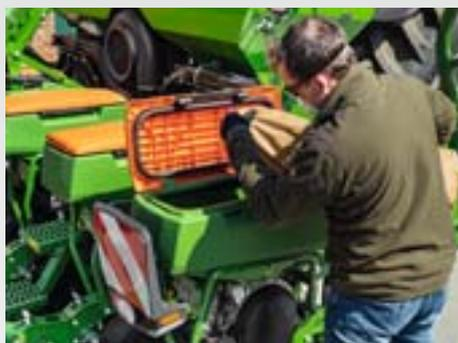
The seed hoppers hold 55 l. The pressurised tanks can be opened with one hand and are protected by a rubber lip against dust ingress. Furthermore, the hopper lids have a chute for removing the residual seed.
