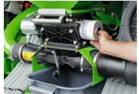
The metering unit of the AD-P Special is driven electrically allowing calibration by the press of a button and the very simple adjustment of the seed rate from the tractor cab. The easy accessibility simplifies the exchange of the metering cassettes and calibration.
