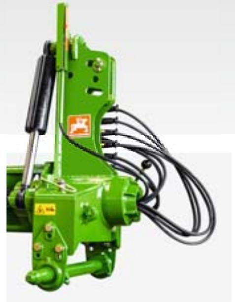
The headstock is equipped with a one-piece lower link cross shaft which has very good shock absorbing properties and in this way significantly reduces the load on the tractor's rear lift linkage. This is enabled by two pivot bearings, one on each side of the lower link cross shaft, which effectively absorb the shock loads generated.
