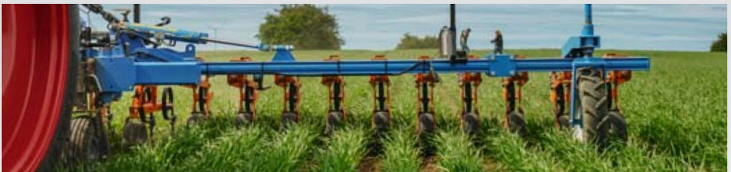
Low wear, e.g. by using HD versions of the soil-engaging metal, is becoming ever more important for hoe systems, due to increasing driving speeds and increasing work rate requirements. In order to decrease the length of time not working, or to simplify blade changing to suit different operating conditions, for example, a quick change knife system is becoming more and more considered as standard equipment. Maintenance-free bearings on the hoes also reduces machine downtime.
