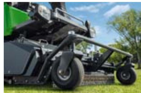
Via the adjustment handle, positioned on the mowing deck of the Profihopper 1500 SmartLine, the height of cut can be adjusted from 0 – 90 mm. Here, the total mowing deck is swivelled so that no parts are positioned deeper to impact the quality of work.
