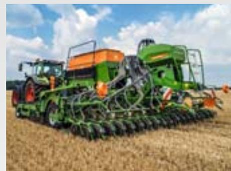
The GreenDrill 501, with 500 l hopper capacity, is suitable for sowing catch crops, fine seeds, undersown crops and spreading fertiliser in combination with the trailed AMAZONE soil tillage range or the Cirrus trailed drill combination.
