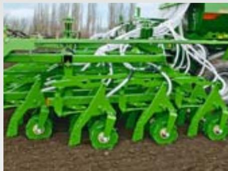
The 4-stagger arrangement of the opener units on the frame results in a large spacing between the openers to ensure excellent straw passage.
