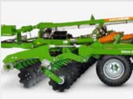
The front discs distribute the organic matter by intensively cutting and mixing the crop residues on the soil surface. At the same time, a finely crumbled structure occurs within that top soil layer.
