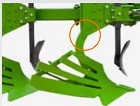
The shear bolt is the proven standard solution for stone safety. Under load, the shear bolt snaps off at the predetermined breaking point and the plough body gives way to the obstacle by swivelling upwards. This means that the plough can also be used in heavy and hard soils.
