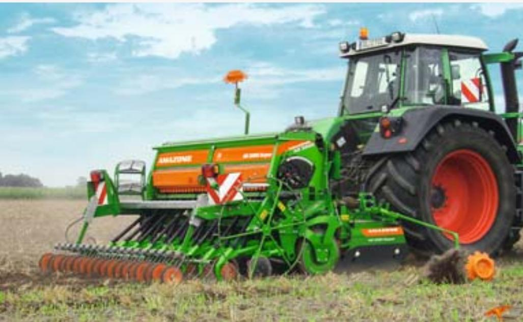
AD 3000 Super, 3 m working width with roller harrow
