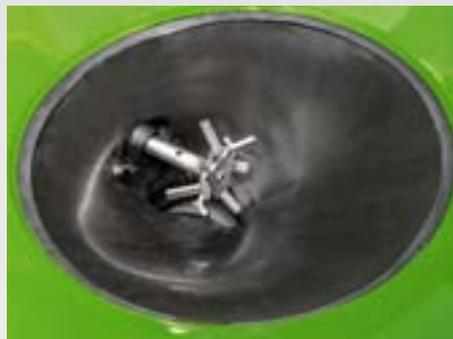
The mechanical star agitator of the ZA-V is positioned directly above the deep aperture and in this way provides a reliable and consistent fertiliser flow at all application rates. Turning at just 45 rpm, it makes for a fertiliser-protecting operation.
