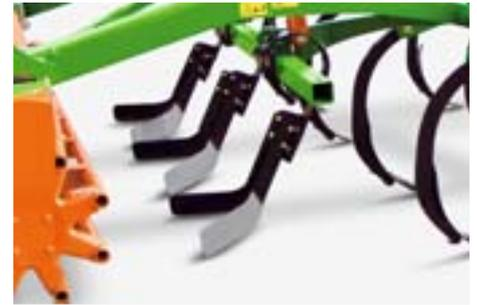
For operation on light soils with little straw prevailing, the Cenius can be equipped with spring closers.
