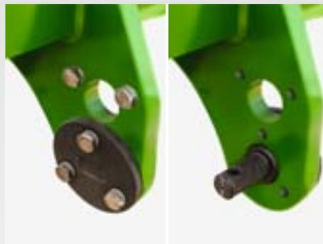
When attached to the tractor, the machine is coupled to the lower links via Cat. 3 pins. However, by simply reversing the pin in the lower link journal, a spacing of either Cat. 3 or Cat. 2 can be achieved.
