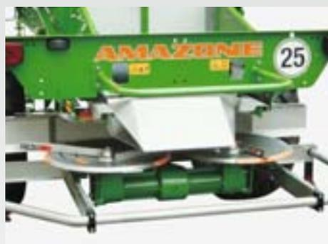
The ZG-B models have a universal spreader unit for the application of earth-moist materials (lime) up to 15 m and mineral fertilisers up to 36 m spreading width.
