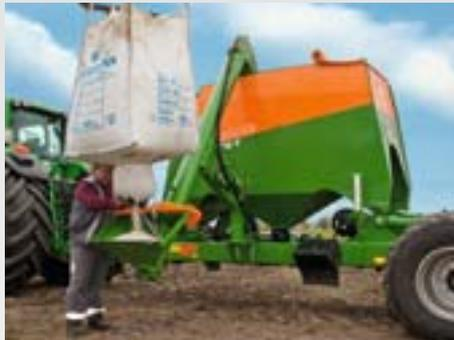
The large openings enable the problem-free filling of the hopper via a front end loader. However, on request, the machines can also be equipped with a filling auger.
