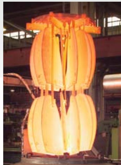
One specific quality feature of the Cayros ploughs is the heat treatment with the ©plus hardening process for the mouldboards. This heat treatment results in a prolonged longevity, high impact strength and a smaller pulling power requirement and thus reduced fuel consumption.
