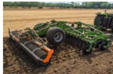
To ensure an even depth control of the machine, the Certos-2TX is guided at the rear via the following roller and up front via the support wheels.
