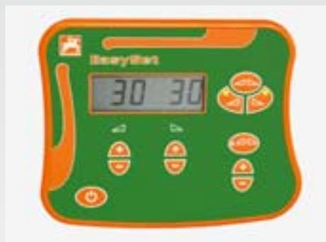
With the aid of the EasySet operator terminal, the spread rate shutter apertures can be electrically set via key pressure independently of each other to either side and can be readjusted on the move. This also allows the rate to be individually adapted to the left and right hand side.
