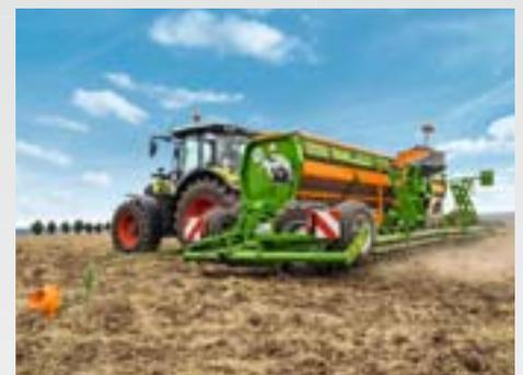
The D9 6000-TC "Combi" trailed seed drill with a 6 m working width is perfect for precise behind-the-plough and mulch sowing. High surface area coverage is guaranteed with a tank capacity of 2800 l for fertiliser and seed and working speeds of 15 km/h.
