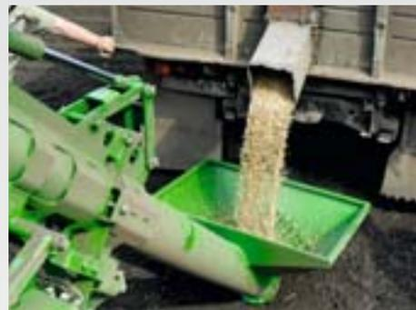
In order to be able to fill the Primera DMC with both seed and fertiliser, AMAZONE offers a hydraulically-driven filling auger. Using this system the filling time is kept down to just 15 minutes meaning that the output of the drill is even further extended.
