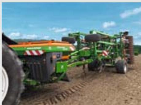
Via the 3-point linkage (Cat. 3/4N), the XTender is mounted onto the tractor with a favourable centre of gravity. The coupling of the following implement onto the Xtender is also carried out via a standardised Cat. 3 or 4N lower linkage
