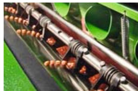
On all EDX machines, the adjustment of the stripper fingers is carried out simultaneously for all the rows. As a special option, electric remote control of the stripper finger is available, enabling the driver to regulate the stripper finger position via the AmaTron 3 in the tractor cab during operation.
