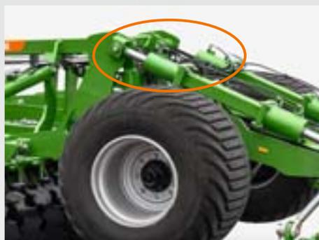
The angle of inclination of the Certos can be adjusted by means of a hydraulic upper tie bar. If the machinery pulls to one side, it can be easily compensated for from the driver's seat in the tractor cab.
