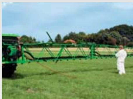
After the spraying operation is finished, with the aid of the spray lance on the wash down kit, any sprayer from AMAZONE can be thoroughly cleaned externally in the field.
