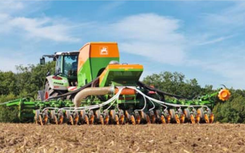
EDX precision air seeder, 6 m working width
