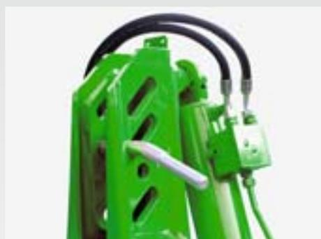
All headstocks come equipped with an elongated hole for the top link. Using this elongated hole position, the tractor/plough combination follows the contours in uneven ground especially well ensuring that the desired working depth is always maintained.
