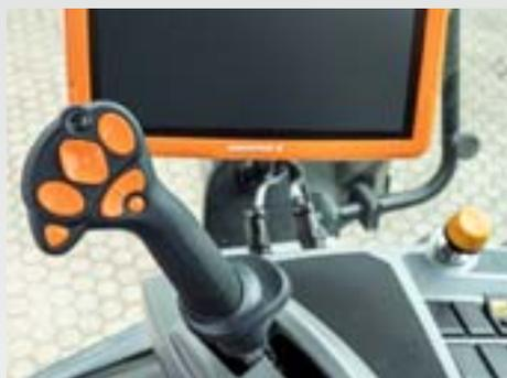
Via the AmaPilot multi-function joystick and the AmaPad 2 operator terminal, the Pantera offers a comfortable and simple operation.
