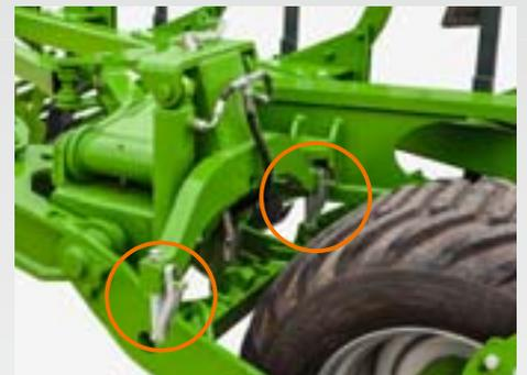
The setting of the plough tilt is done without tools and is adjustable individually for the right and left hand side.
