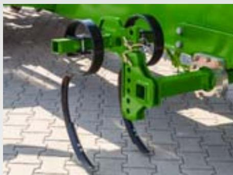
For operation on loose or poorly reconsolidated soils, wheel mark eradicators are available as option. The wheel marks are loosened and levelled. By hydraulic actuation, the lowering and lifting is carried out automatically on the headland or when folding for transport.
